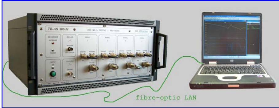
TR-AS® RC with 1 to 4 measuring channels located closed to the test field
