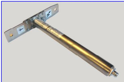
The Impulse Current Measuring Shunts ICMS are designed for measurements of impulse currents with shape 8/20  $\mu$ s according to IEC 60060-1. For impulse currents with any shape the maximal action integral or the maximal voltage drop must not be exceeded.
